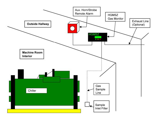
**HGMSZ Refrigerant Gas Leak Monitor Mechanical Room Placement**
